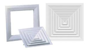
These are used for air supply in multiple layers which help to speed up induction of secondary room air thus assuring draft-free comfort in occupied spaces. Four-way square diffusers give equal supply in all directions while throe, two and ono diffusers limit the supply in tho required direction. Removable core simplifies installation and avoids visible mounting screws.
