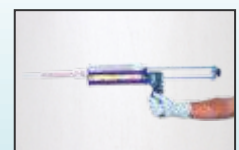
5. Screw mixing nozzle onto cartridge and dispense 2-3 trigger pulls of adhesive to waste until color is red with no streaks.
