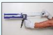
3. Pull Injector out at maximum range.
