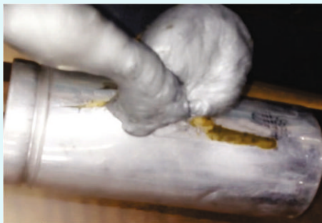
TYPICAL PICTURE OF A BURST CAPACITOR
